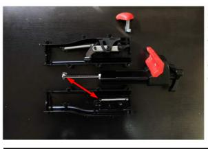
Disassembled view: Note that tension spring is disconnected from chrome hook end of sliding clamp assembly (left).
