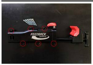
Step 3: Remove six 4 mm allen bolts on side of clamp body.
