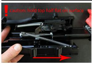
Step 6: While holding both body halves, gently pull spring to align body halves. Take care to not pull internals out of upper half with spring.
