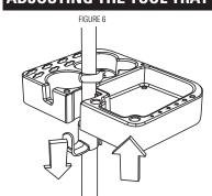
NOTE: To reposition, lift Tool Tray half way off the Tray Mount, slide the tray Mount to new Position and push Tool Tray back down onto Tray Mount.
