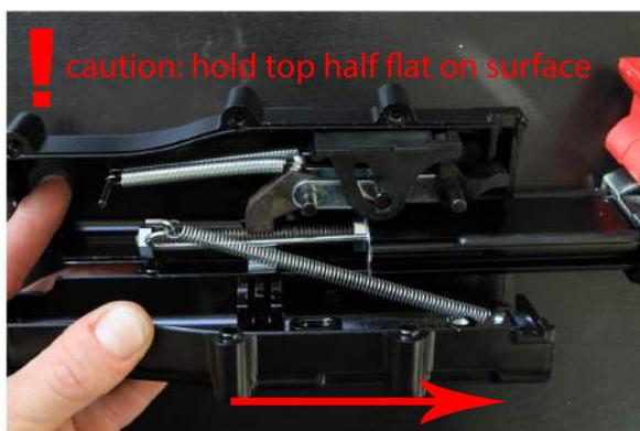
**Step 6:** While holding both body halves, gently pull spring to align body halves. Take care to not pull internals out of upper half with spring.
