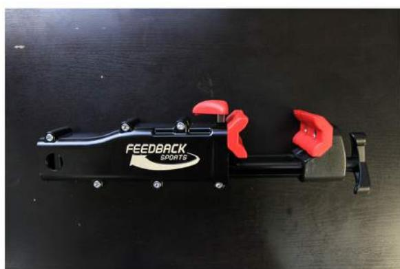
**Step 9:** Reinstall inner clamp jaw with two 4mm allen bolts.
