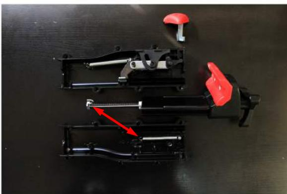
**Disassembled view:** Note that tension spring is disconnected from chrome hook end of sliding clamp assembly (left).
