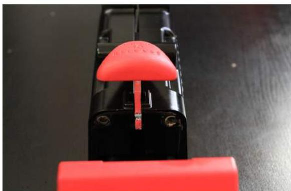
**Step 7:** Slide clamp release button into channel between body halves then gently press body halves together.
