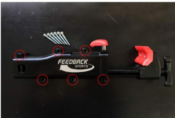
**Step 3:** Remove six 4 mm allen bolts on side of clamp body.
