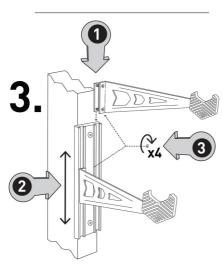
NOTE: After mounting the wall rack and adjusting the arms, tighten all screws. Test by weighting with equipment to insure proper installation. Feedback Sports is not responsible for any damage resulting from improper installation.
